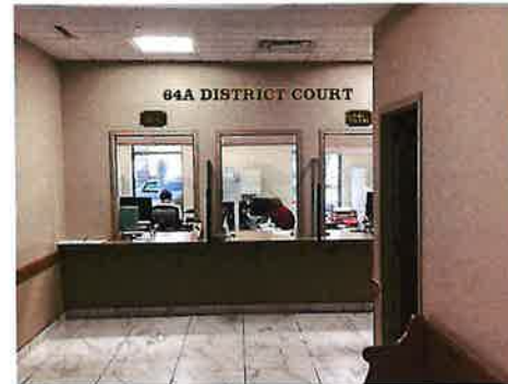
3/8" THICK ACRYLIC LETTERS w/ SATIN PAINTED FINISH MOUNTED FLUSH TO WALL, 1/8" THICK ACRYLIC PANELS w/ RAISED GOLD LETTERING MOUNTED FLUSH TO WALL
