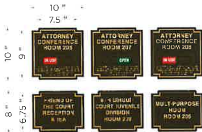
1/8" THICK ACRYLIC PANEL w/ RAISED GOLD LETTERING & BORDER, RAISED BRAILLE & (3) WITH SLIDER FOR ROOM USAGE, MOUNTED FLUSH TO WALLS
