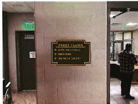
1/8" THICK ACRYLIC PANEL w/ RAISED GOLD LETTERING & BORDER MOUNTED FLUSH TO WALL
