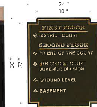
3/8" THICK ACRYLIC LETTERS w/ SATIN PAINTED FINISH MOUNTED FLUSH TO WALL, 1/8" THICK ACRYLIC PANELS w/ RAISED GOLD LETTERING MOUNTED FLUSH TO WALL
