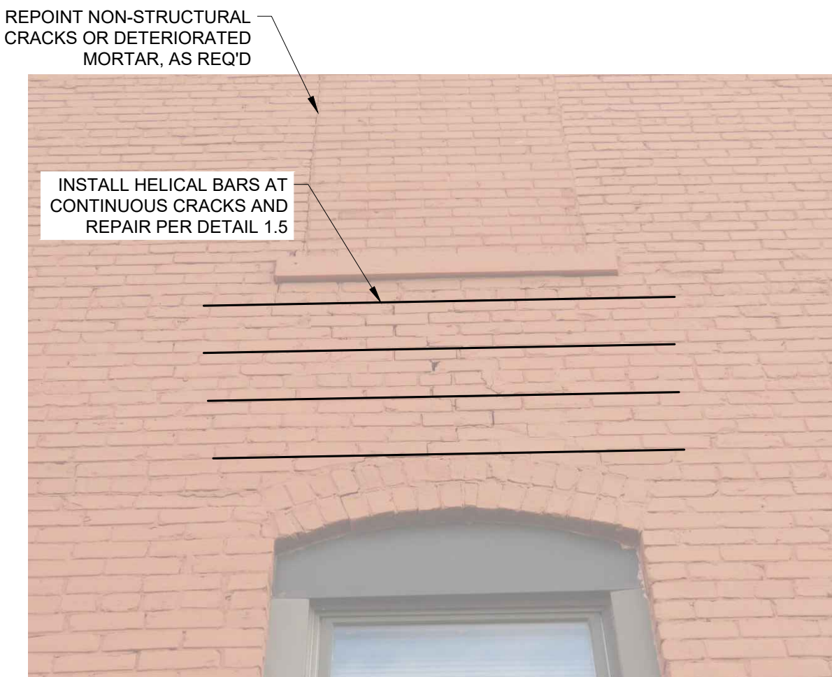
1.3 Masonry Crack Stitching Repair, Typ.
